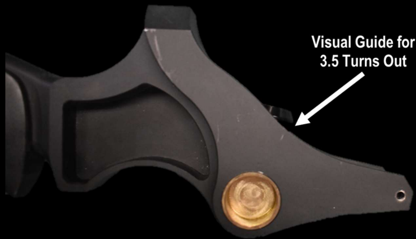
Figure 9 Three Turns Out Condition
