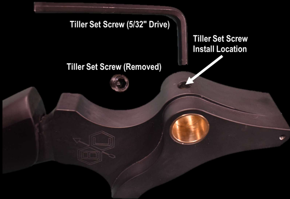
Figure 9 Tiller Set Screw
